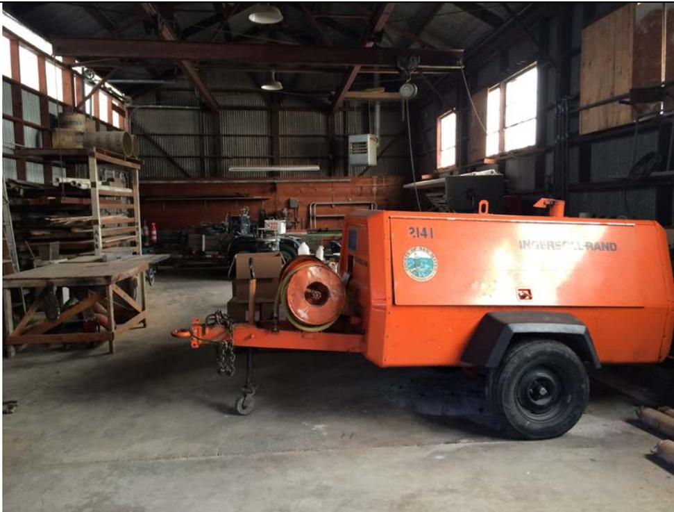
Photo 6: Twenty-four-gallon diesel-powered mobile air compressor located in the carpentry room of the building located along the southern Site boundary.
