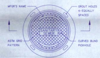
\* ALL MATERIALS USED SHALL CONFORM TO ASTM SPEC. A-159-70T-03000 OR U.S. GOV'T SPEC. Q01-653
